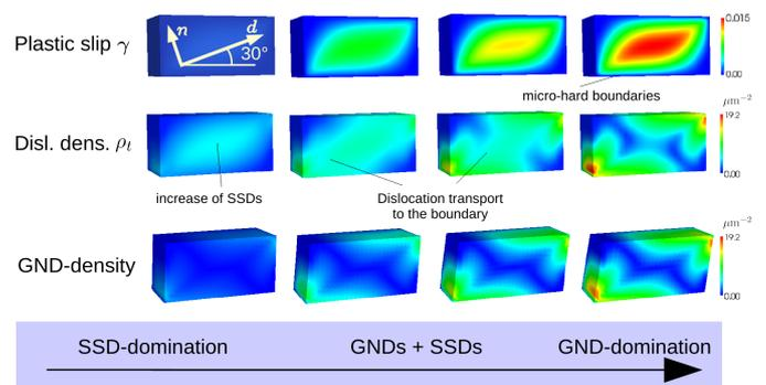
Fig. 3 FE-Simulation of the simplified kinematical theory and comparison with GND-theory. Only the backmost half of the single crystal is represented to visualize the fields in the single crystal.
