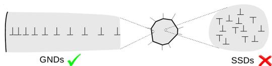
**Fig. 1** Schematical representation of a dislocation pile-up and a typical SSD-configuration; while the first mechanism is well-represented through  $\boldsymbol{\alpha}$ , the SSDs are “invisible” using this dislocation density measure.
