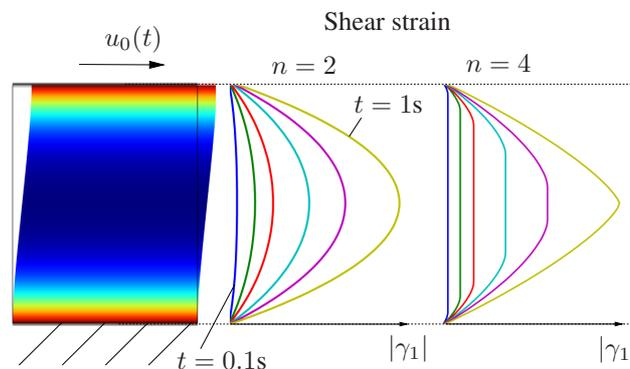
**Fig. 3** Evolution of the absolute value of the plastic shear strain  $|\gamma_1|$  for  $n = 2$  and  $n = 4$
