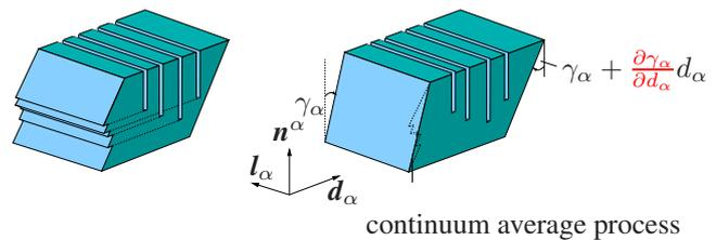
**Fig. 2** Typical GND-example: several parallel edge dislocations of equal sign lead to a non-vanishing strain gradient
