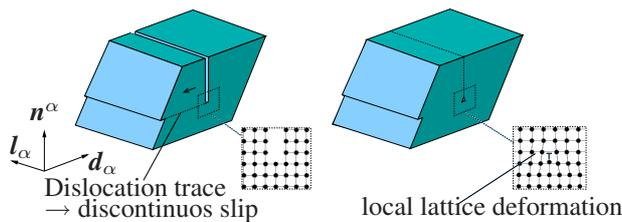
**Fig. 1** Introduction of a discrete dislocation into a homogeneously deformed single crystal
